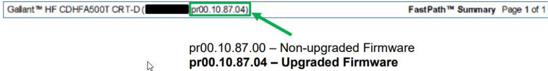
Image 1: Firmware version displayed in the footer of a Merlin™ PCS 3650 or Merlin™2 PCS programmer reports
